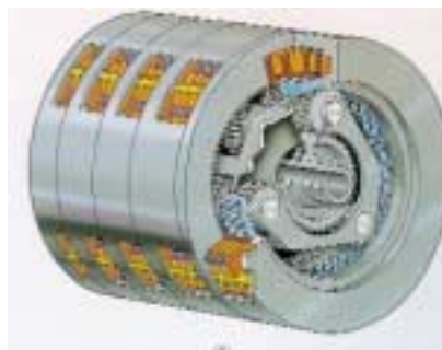
Inside transmission with planetary gears
