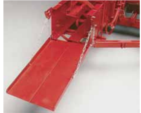
Triple-purpose chute supports bales as they leave the chamber; can be set to roll bales to left, away from next windrow. (Also becomes the base for bale-loading chute.)
