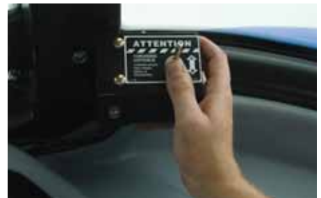
Distance and direction controller attaches to the tractor. The toggle switch controls the speed of the throwing belts for distance.
